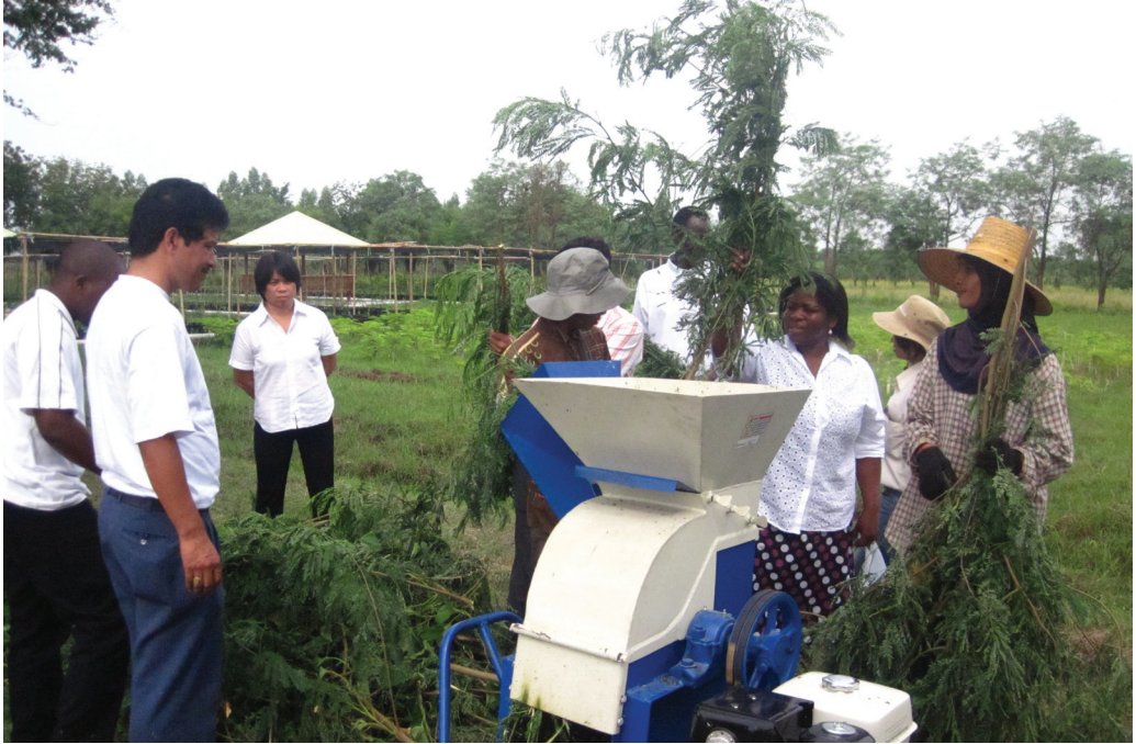
Figure 6. Chopping compost materials using a motorized shredder.
