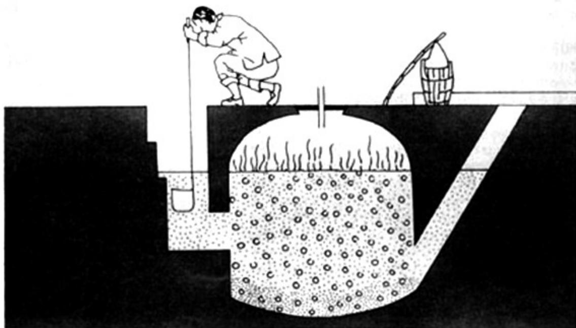
Plate 31 Removal of biogas sludge from the sludge outlet pipe Source: FAO filmstrip Biogas in China
