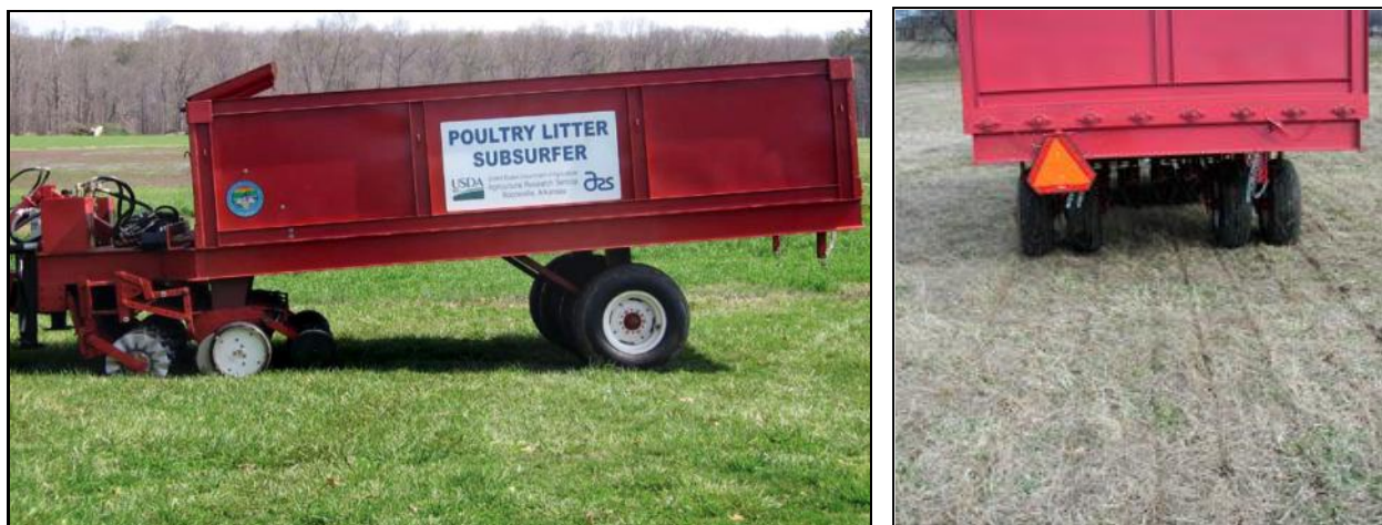
Figure 6. Left: USDA's Agricultural Research Service demonstrates a prototype poultry litter subsurfer in Arkansas. The subsurfer is designed to apply litter under the surface of perennial pasture and other no-till systems, and gives farmers precise control of litter application rates. Right: Subsurfer leaves a "clean" soil surface after application. Photos by Stephanie Jordan.
