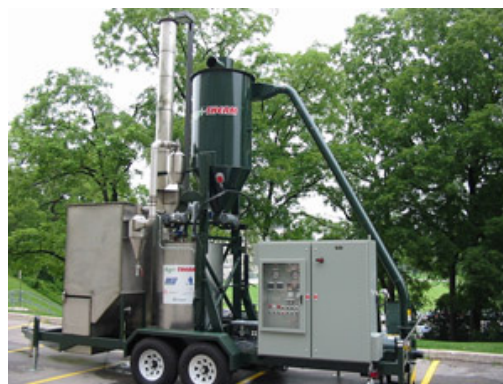
Farm scale mobile pyrolysis unit from Agritherm.
