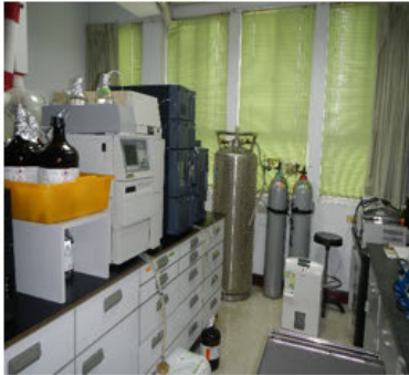
Laboratories: Gas Storage in poorly ventilated instrumentation rooms – toxicity and asphyxiation hazards (especially liquid nitrogen).
