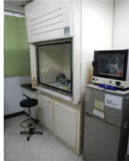
Laboratories: Poor ergonomic design around fume cupboards and other major equipment.
