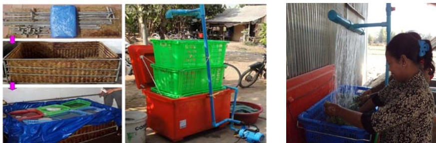
Figure 22 Simple knockdown hydrocooler (leftmost) and overhead hydrocooler applying cold water with water pump on the produce (middle and rightmost).
