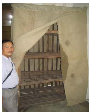
Figure 24 Brick-walled and box-type evaporative coolers (EC).
