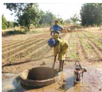
Female farmers use a rope and bucket ( right ) and operate a treadle pump ( left ) to draw water from wells to irrigate their vegetables
