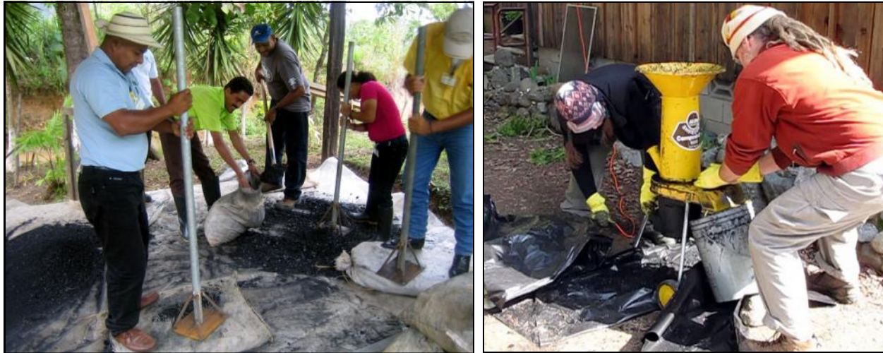
Figure 1. Left: Hand crushing biochar inside sacks in Honduras. Photo by J. Major. Right: Crushing moistened biochar using a small compost shredder in Oregon, USA. Photo by D. Dalegowski.
