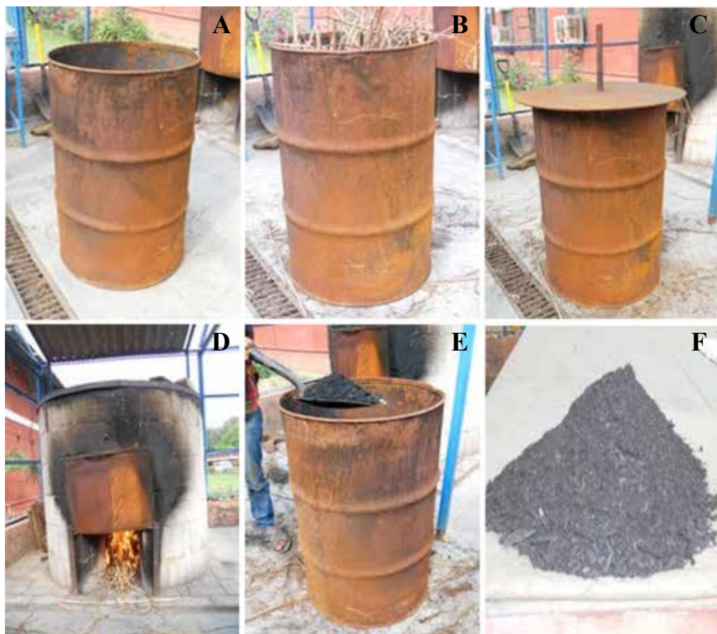
Biochar preparation at IARI: Drum used for preparation of biochar (A); Drum filled with maize stover (B); Drum covered with lid (C); Drum placed inside the firebrick kiln heating provide at the base of drum externally (D); Biochar removed from drum (E); and Biochar the final product with little percentage of ash (F)
