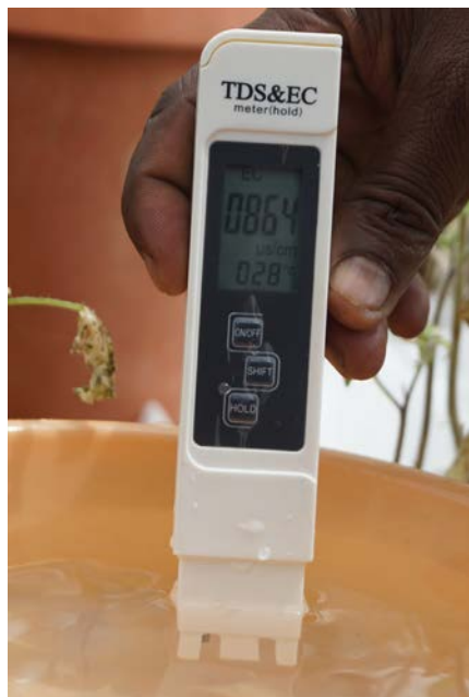
Figure 39: Measuring EC of the medium
