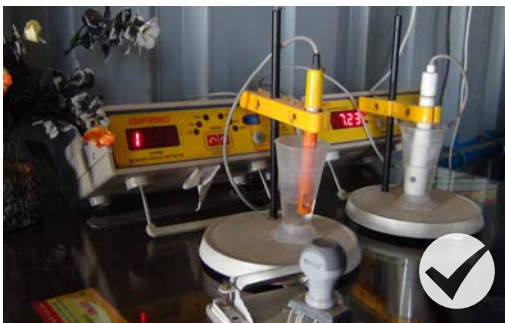
Install EC meter and pH meter
