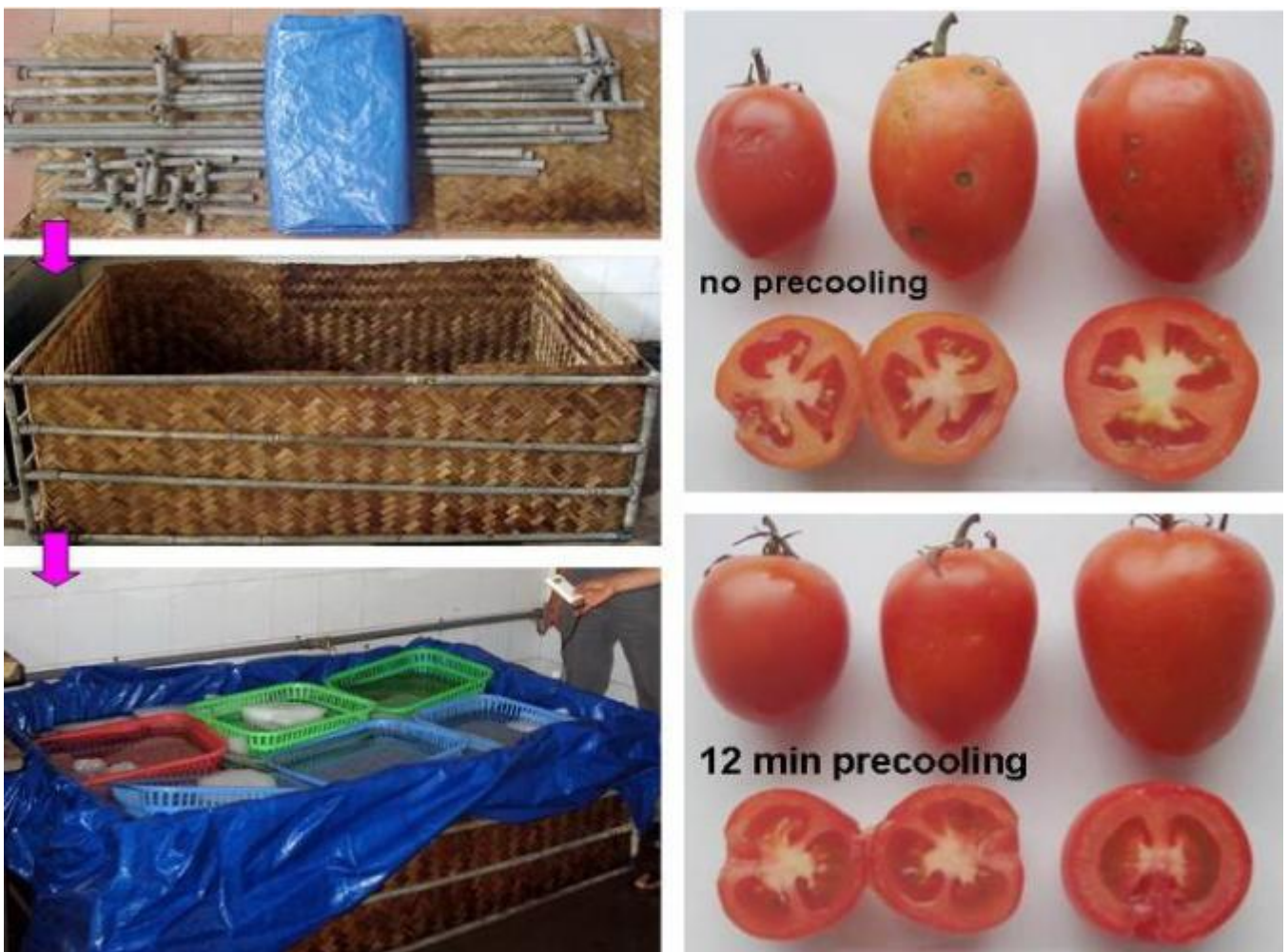
Simple hydrocooler for vegetables and fruit developed at FAVRI, Vietnam, and its effect on reducing tomato chill injury (brown spots) in 10°C storage.
