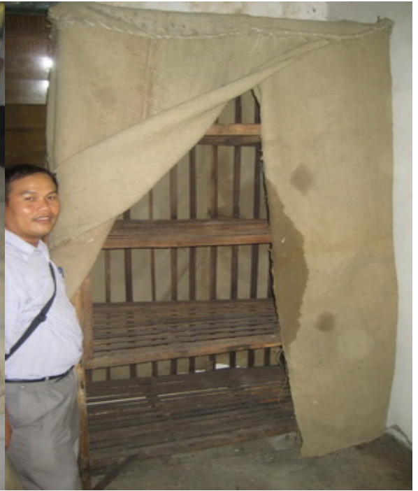
Box-type EC 1.3x0.9x2.0 m in L, W, H, with moist jute sack
