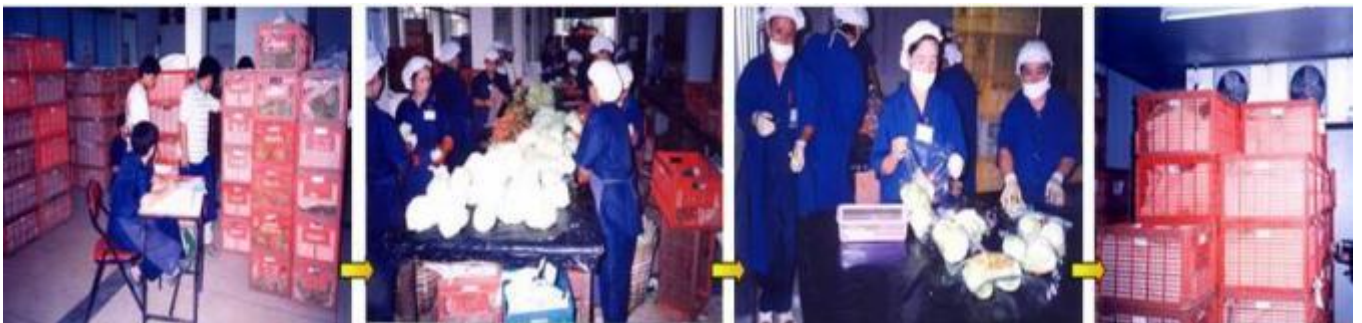
Packinghouse activities for cabbages for supermarkets: produce arrival recording-wrapper leaf removal, butt trimming and lime application for soft rot control-plastic film packing-crating-precooling and storage
