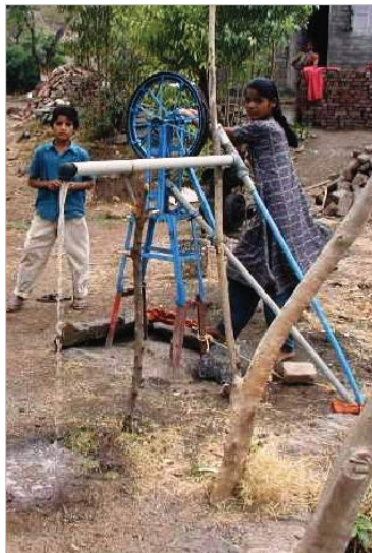
Figure 15. Drawing water from well with a manually operated rope pump.
