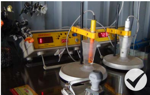
Install EC meter and pH meter
