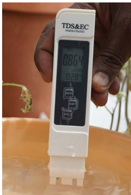
Figure 39: Measuring EC of the medium
