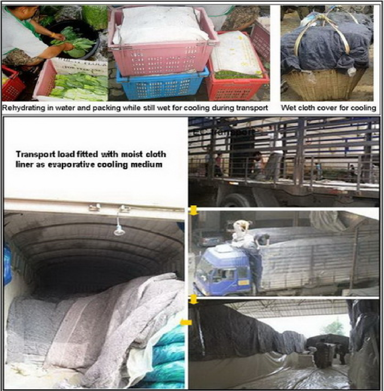
Evaporative cooling (use of wet cloth) and MA film liner in transport load.
