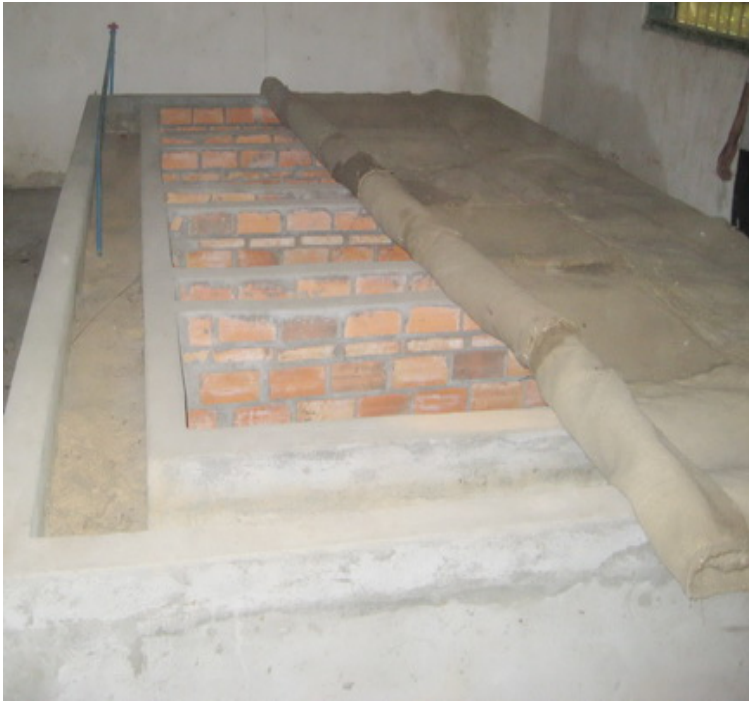
Brick-walled EC 4.5x2.5x0.6 m in length, width & height, 15-20 cm double wall with moist sand
